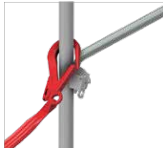
Fig. 93: Limit stop at the stand above the upper guard rail
