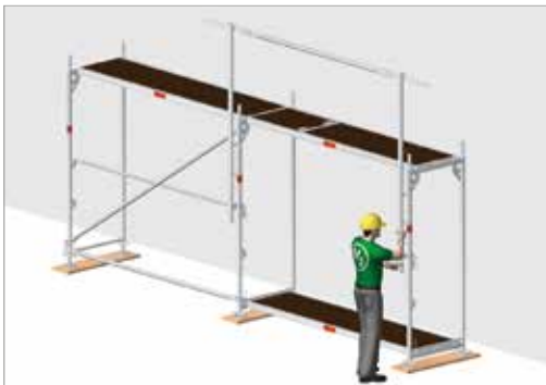
Fig. 88 Installation of the second MSG post
