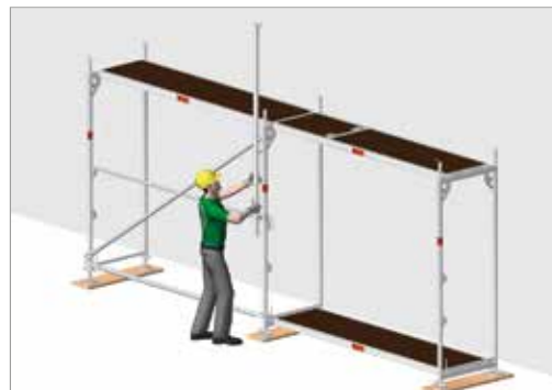
Fig. 85: Installation of the first MSG post
