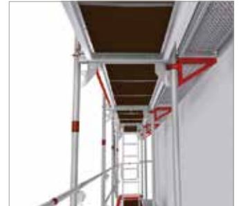
Fig. 54: Level of the inside brackets
