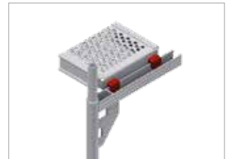
Fig. 15: Hooked-in system deck, located inside near displacement protection
