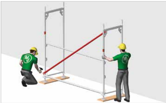
Fig. 11: Assembly of the first scaffold field: Vertical diagonal
