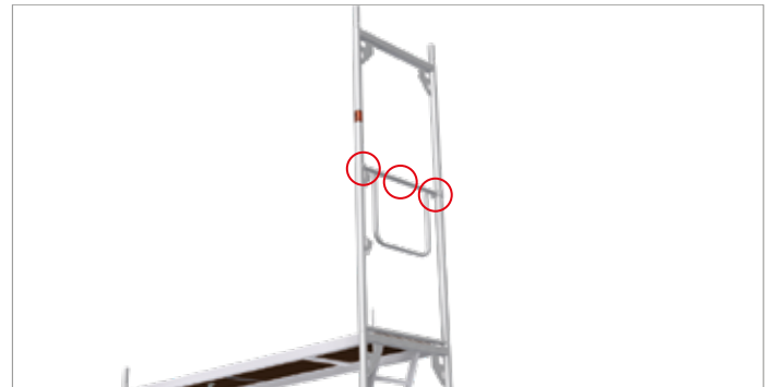
Fig. 95: Admissible anchor points for the PSaGA at the front railing above a stand height \geq 6 m
