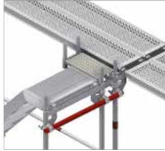
Fig. 37: Connection to the main frame through scaffold tubes and couplers
