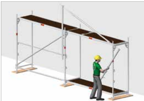
Fig. 87: Insertion of the MSG guard rail stringer at the second MSG post
