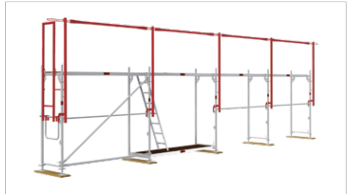
Fig. 25: First scaffold level with surrounding assembly security guard rail (MSG)
