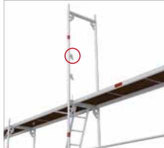
Fig. 99: Admissible anchor point for the PSAgA at the guard rail wedge housing above a stand height \geq 6 m
