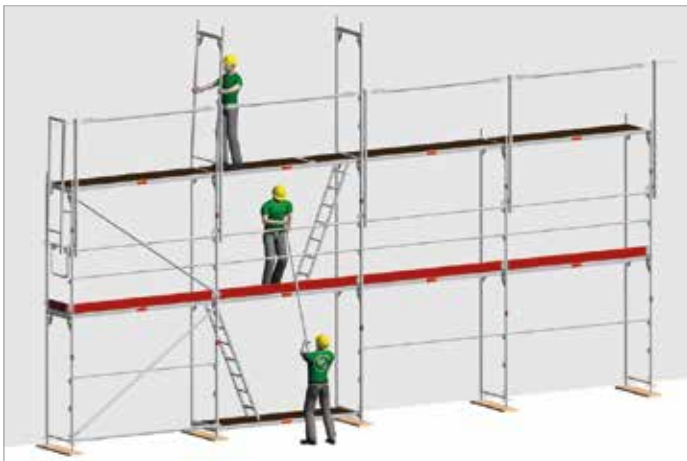
Fig. 26: Installation of further scaffold levels under cover of the MSG
