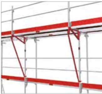
Fig. 56: Scaffold with outside 0.73 m brackets and bracket struts in uppermost level
