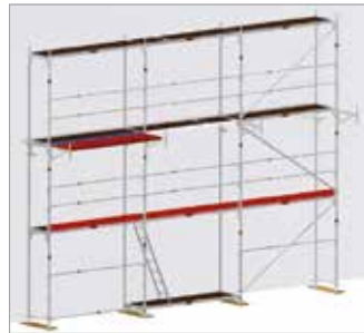
Fig. 60: Insertion of the system decks into the 0.73 m brackets, alum. intermediate deck as a gap cover
