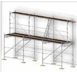
Fig. 74: Scaffold section with walk-through frames and braces, as well as anchors at height H = 4 m, installation of the second level
