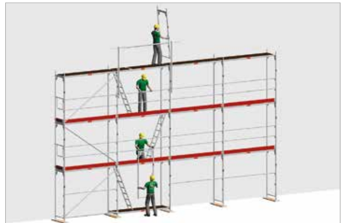
Fig. 31: Ascent field assembly under cover of the MSG
