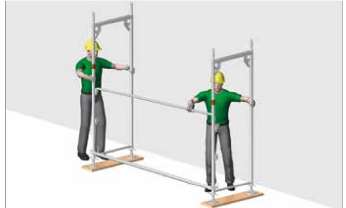
Fig. 8: Assembly of the first scaffold field: Guard rail, horizontal brace
