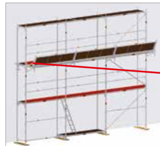
Fig. 66: Scaffold with 3-part side guard in the area of the roof guard
