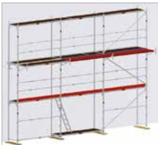
Fig. 61: Installed system decks and gap covers
