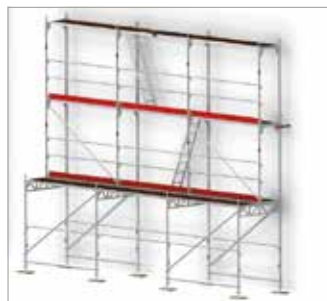
Fig. 75: Scaffold section with DGR and side guard; installation of the further level
