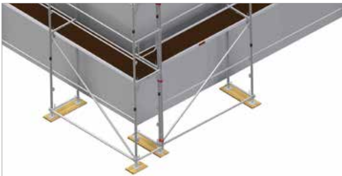
Fig. 19: Corner formation of the lowest scaffold level
