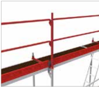
Fig. 41: Upper close-off of the scaffold with L-shaped guard rail posts, guard rails and toe boards
