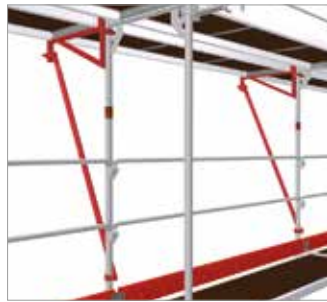
Fig. 57: Connection of the exterior brackets and bracket struts
