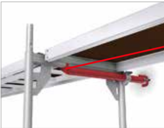
Fig. 44: Wall tie with plate (basic configuration)
