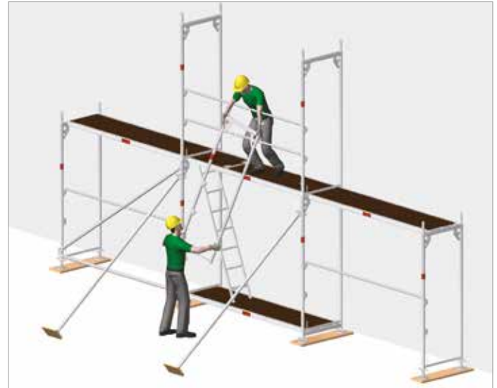
Fig. 2: Example of a temporary tilt protection with installation of the second scaffold level
