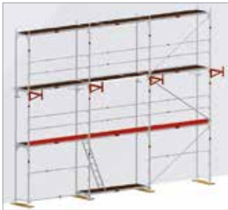
Fig. 59: 0.73 m bracket as a protective roof bracket at the outer side of the scaffold
