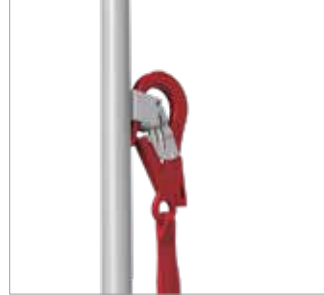
Fig. 100: Limit stop at the guard rail wedge housing
